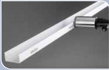
6000RPlus programmed for continuous repeat printing at defined intervals on an extrusion line.
